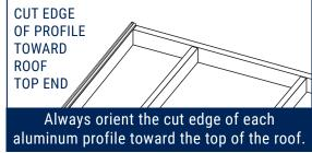
Use a drop saw or angle grinder to cut each profile component to the exact length required.
