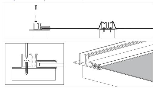
Start fastening the Edge Bottom Glazing Bar to the timber structure using the 8G x 50mm at the bottom of the roof line, and work towards the top. Use the Spacer to make sure the Edge Bottom Glazing Bar is at 600mm centres. 10 Install the Edge Middle Glazing Bar on either the left and right side Edge Bottom Glazing Bar.
