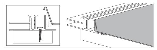
13 Installing Left and Right Edge End Cap and Cap Covers.
