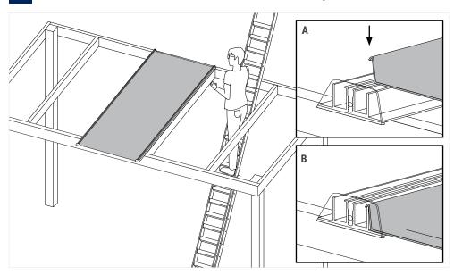
Make sure the raised edges of the Roof Panel are seated along the length of both Bottom Glazing Bars.
