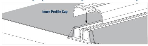
After two adjacent Roof Panels are in place, install a Middle Glazing Bar over the Bottom Glazing Bar between them. This will secure down two adjacent Roof Panel edges.
