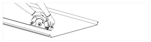
• Bring the sheet to the ground. Cut the Roof Panel along the rip line.
