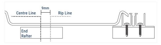
• Set the uncut end Roof Panel in place. On the Roof Panel, note the centre line of the end rafter. Then subtract 9mm and mark that as your rip line along the Roof Panel.
